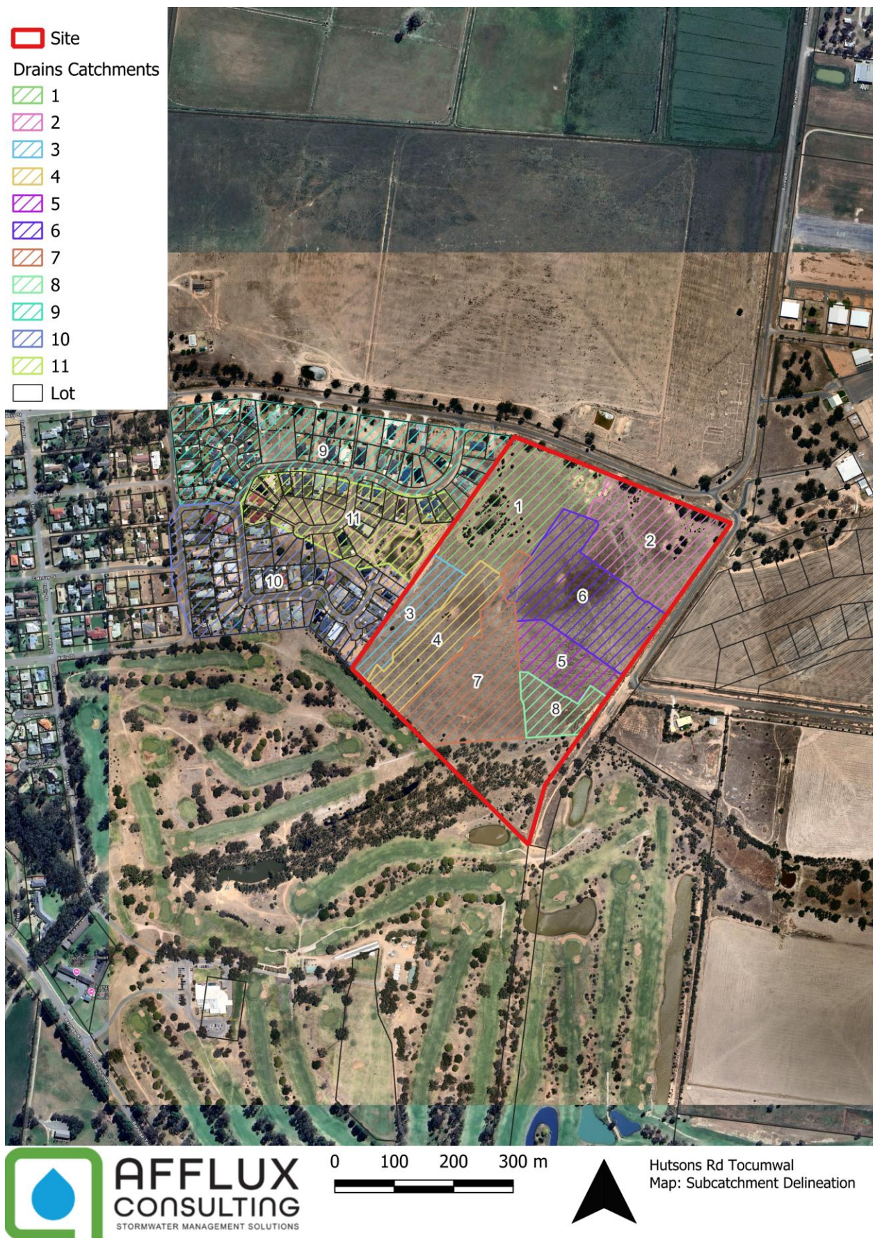
Figure 9. Representation of sub catchment delineation for the DRAINS model
