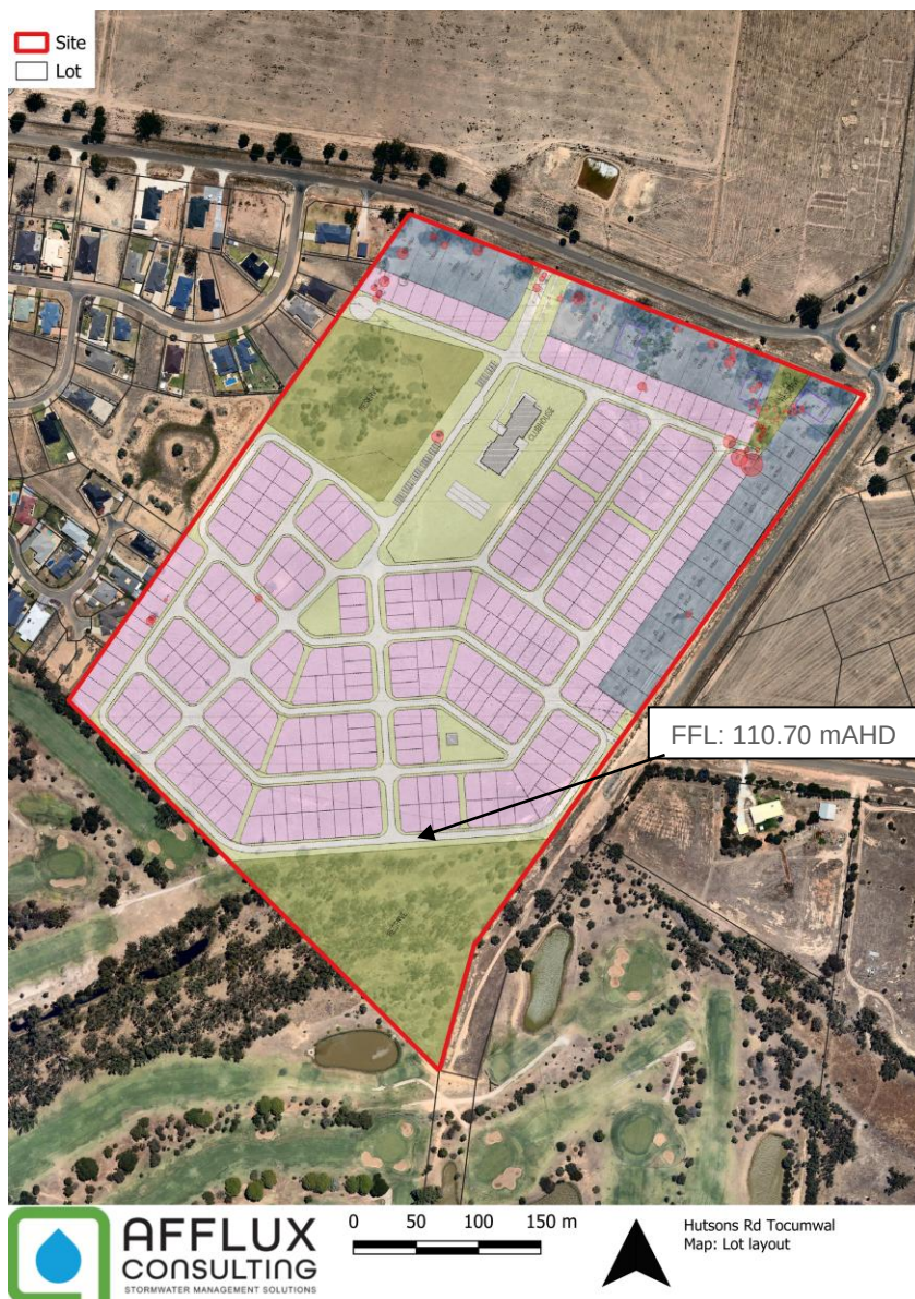
Figure 49. Finished Floor Levels
