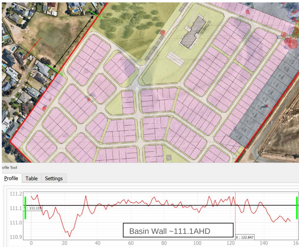
Figure 15. Basin Weir Outfall LiDAR Levels
